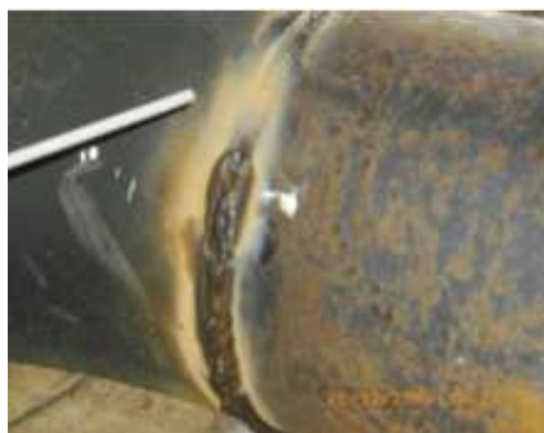
Fig.1: X70 pipeline steel after industrial arc welding
