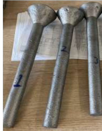
Figure 4. Specimens removed from the sand mold
