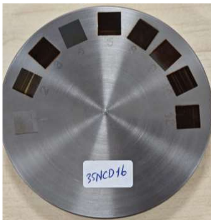
Figure 2.3: Laser induced burns on 35NCD16 low-alloy steel.
