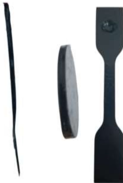
Figure 8. Faulty productions of 1% TiN resin mixture
