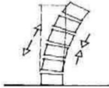
Fig. 2. Behavior of Masonry Elements Subjected to Flexural Action
