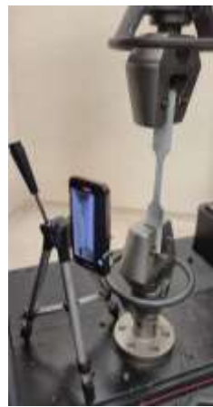
Figure 3. Digital image correlation experiments
