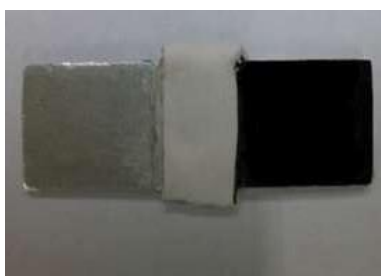
Figure 2: Image of electrode with the PPy coating
