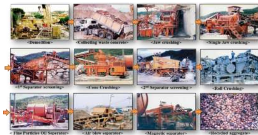
Figure8.ProductionProcessofRecycledAggregate
