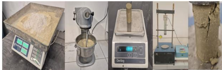
Figure 3. Stages of the Unconfined Compression Test
