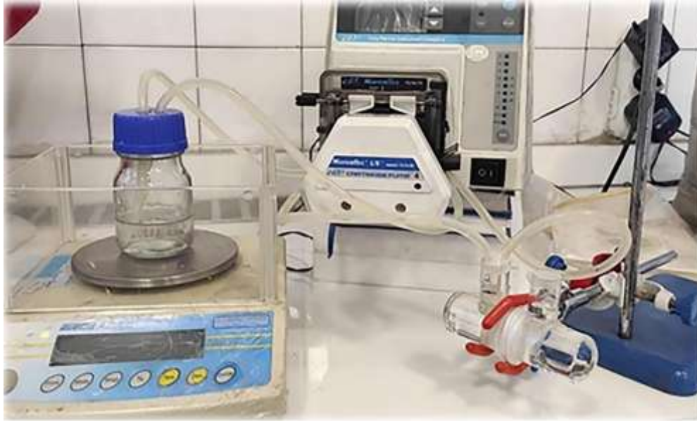
Figure 2.1. FO system (50 rpm; 4.0 M \text{CaCl}_2 \cdot 2\text{H}_2\text{O} )
