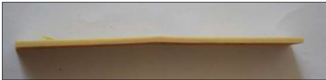
Figure 9: Figure 8: Fractured Compressive Test Specimen (Side view)
