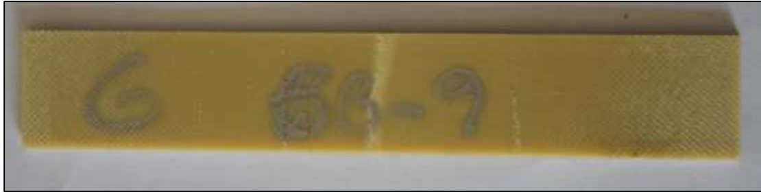
Figure 8: Fractured Compressive Test Specimen (Front view)
