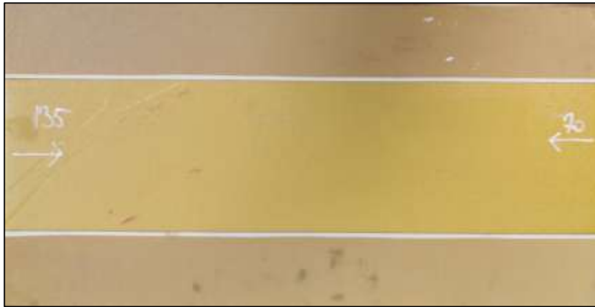
Figure 4: Tab Bonded Tensile Test Laminate
