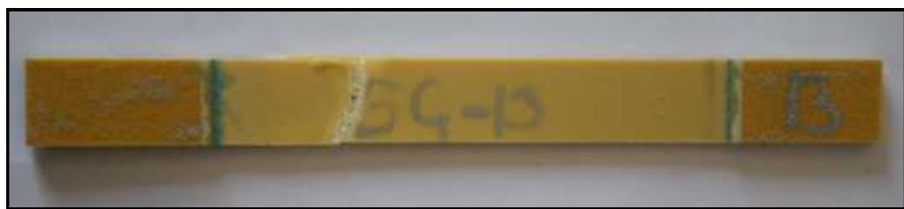
Figure 7: Fractured Tensile Test Specimen
