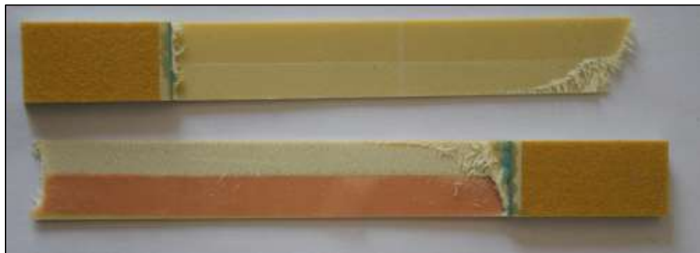
Figure 6: Fractured and Separated Tensile Test Specimen
