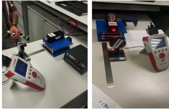
Figure 2. The optical power meter and thermal sensor used for the optical power density characterization
