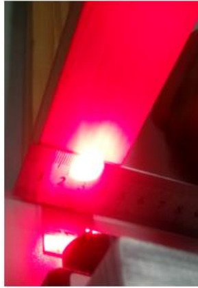
Figure 4. The measurement of diameters of the light spots created by the laser beam
