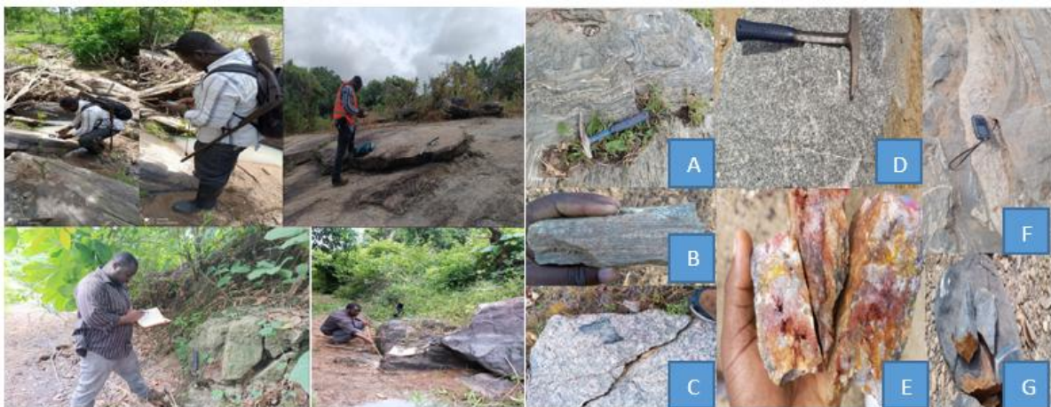
Figure 5: Field Mapping exercise and Hand Specimen Samples of Rock: A: Migmatite-gneiss, B: Gneiss, C: Coarse Grained Granite, D: Granite, E: Altered Quartz, F: Migmatite, G: Amphibolite
